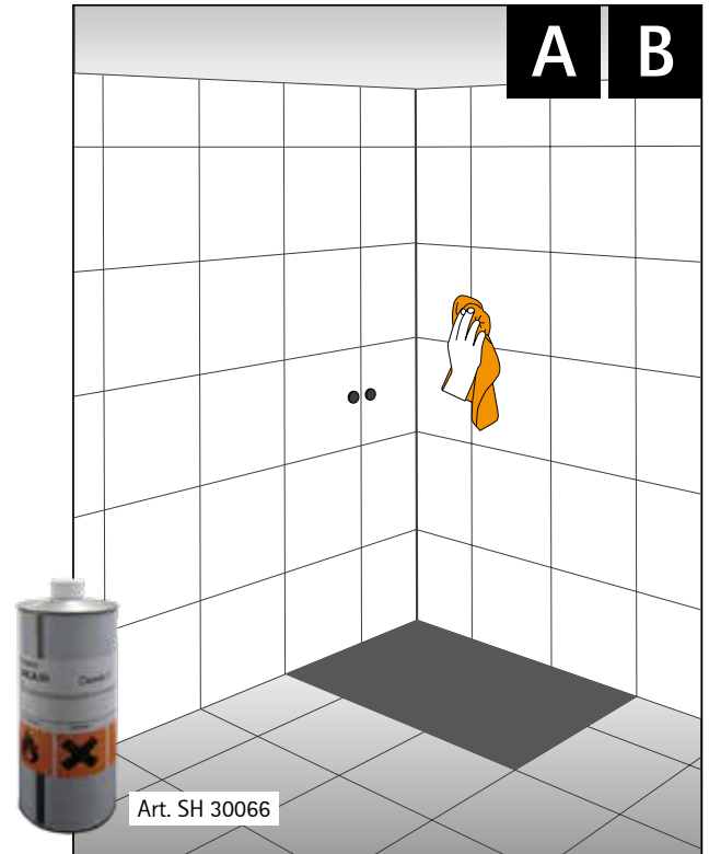
Clean the existing tiles using a soft cloth and our basic cleaner for existing tiled surfaces (Art. SH 30066).
