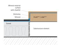
For installations that are not ground-flush, the chamfer provides a jointless, homogeneous surface that includes the shower edge, and thus creates a clean rim to the shower surface.
